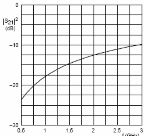
Diode zero biased and inserted in series with a  $50 \Omega$  stripline circuit.
