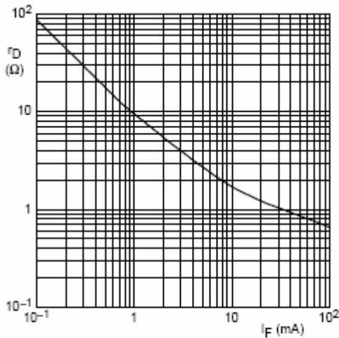
$f = 100 \text{ MHz}; T_J = 25^\circ\text{C}.$
